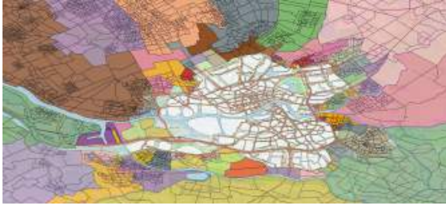
Figure 4.2: Zone layout for the external RODY zones (zoomed in on Rotterdam). White zones are the RODY zones in Rotterdam. All other colours represent a coupling to a VMRDH zone to an external link
