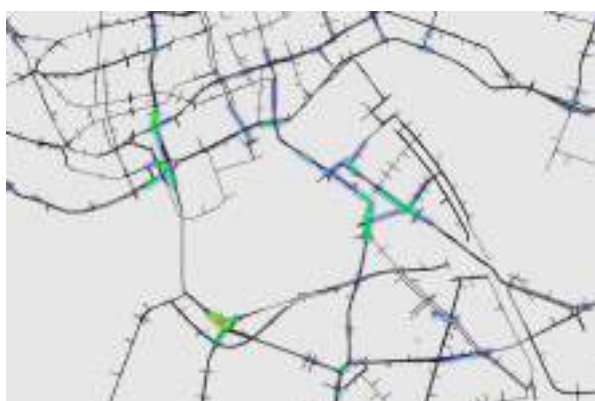
Figure 7.5: Average congestion heat map of Roseknoop roadworks phase 1 as a new equilibrium (iteration 3)
