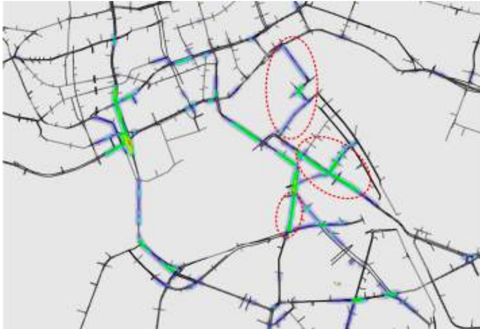
Figure 7.6: Average congestion heatmap of Roseknoop roadworks phase 1 at 5 PM with original OD matrix (no disappearing traffic). Red circles indicate additional traffic congestion locations compared to the congestion heat maps of the new equilibrium.
