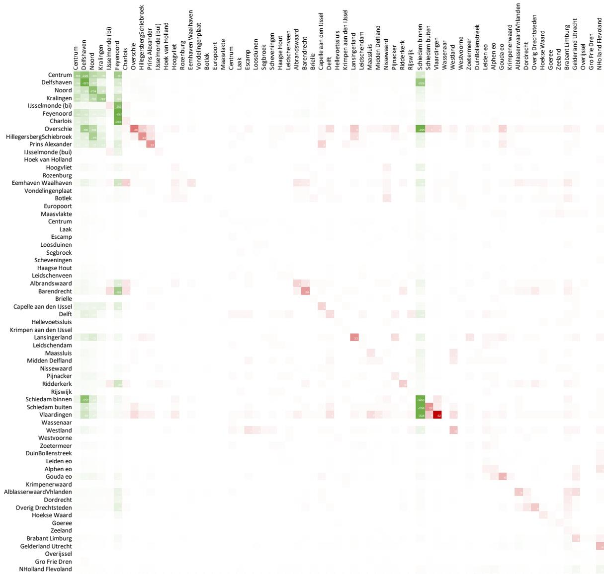
Figure 41: Difference between OD-Matrices BAU and intermediate scenario for mode=car and purpose=all with the modified V-MRDH method.
