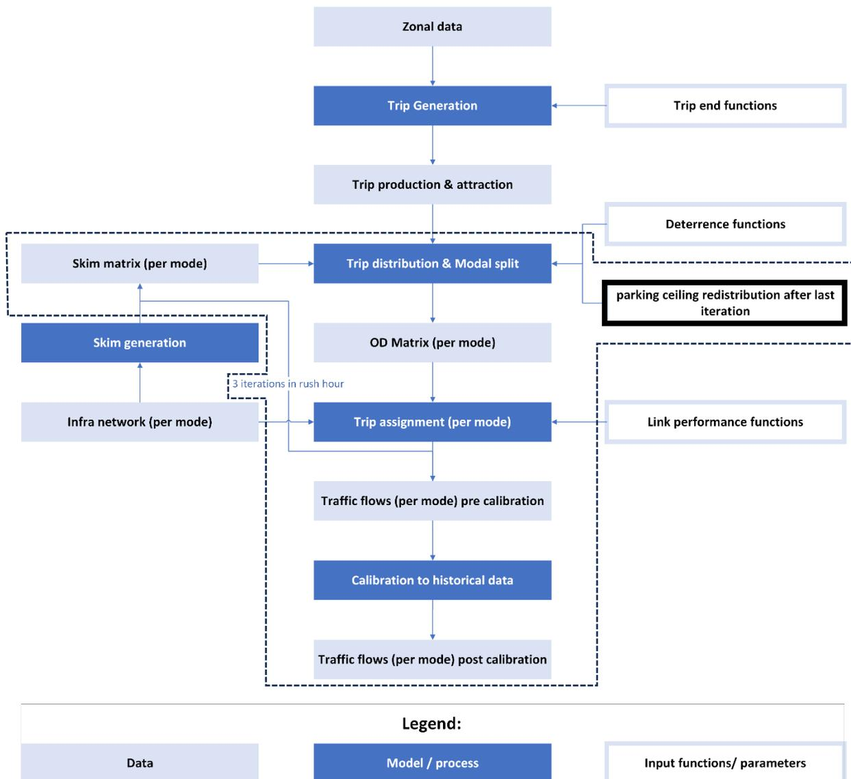
Figure 9: V-RMDH framework adapted from Goudappel, 2023. In solid black the changed input. In striped black the affected steps.
