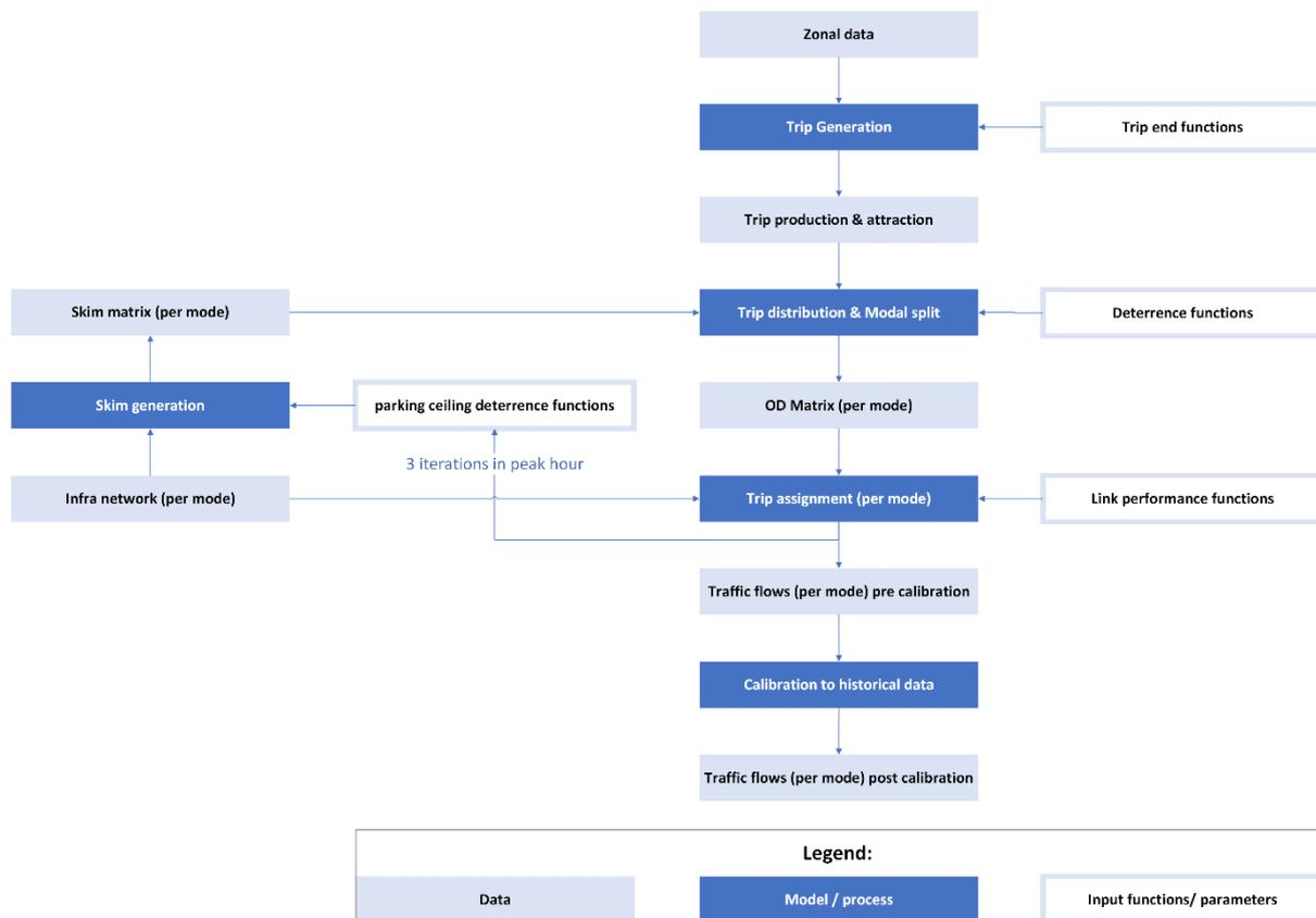
Figure 24: Altered framework V-MRDH model where the parking ceiling is incorporated in the feedback loop.
